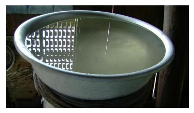
Figure 283: Water inside the top basin. The alcohol vapour will condense quickly on contact with the cold bottom surface of the basin.
