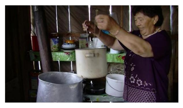
Figure 265: Dolgorsüren suspends a smaller pot inside the top of the distillation column, which will collect the liquor. This is an ordinary enamel over steel cooking pot with string loops affixed to either handle.
