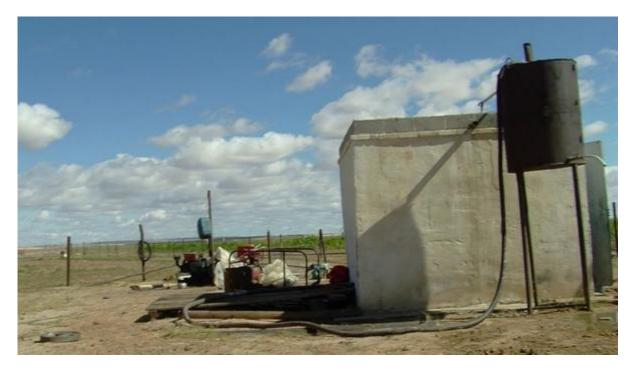
Figure 333: The new reservoir that Delgersaikhan has had installed at the farm. The well inside the building has been drilled to a depth of 80 metres, with the water surface located at 27 metres underground; this well provides one tonne of water per day.
