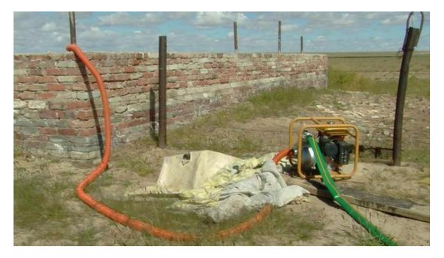
Figure 335: The water pump. Delgersaikhan uses a gasoline pump to draw water from the open reservoir, which then feeds a sprinkler system to irrigate the corn crop.
